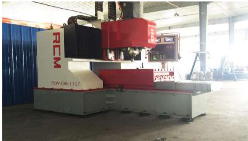
Fig.3. Experimental set up of FSW in BARC
